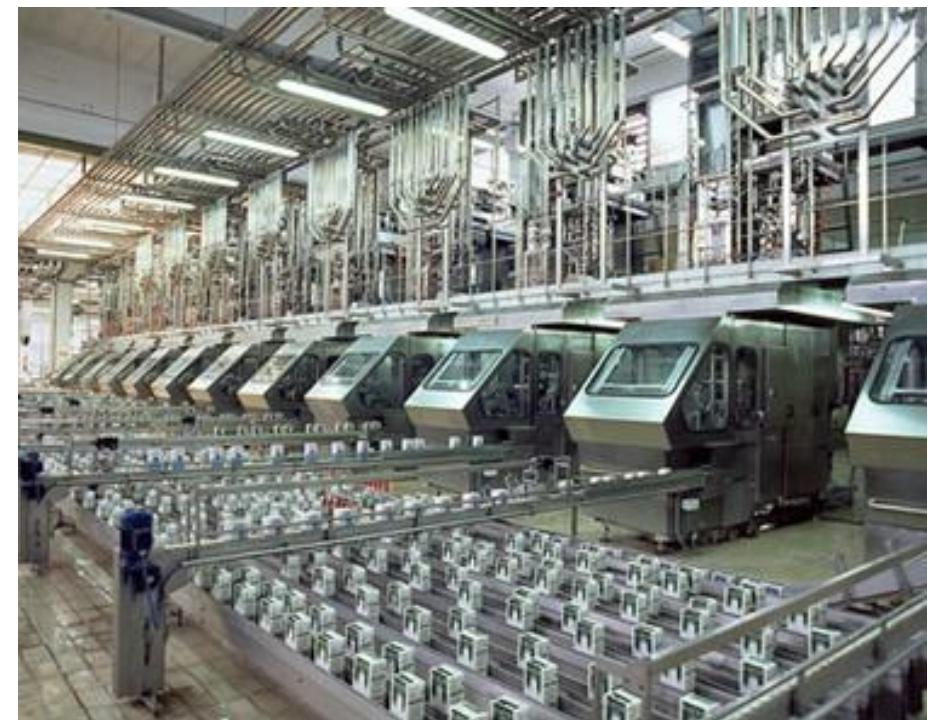
Milk packaging line, 304L stainless steel used extensively
