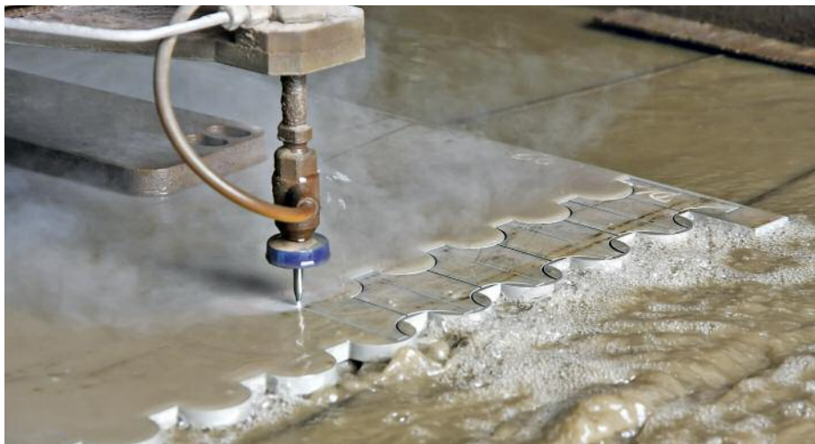
水射流切割不锈钢板。© Lubos Chlubny/Shutterstock.com
