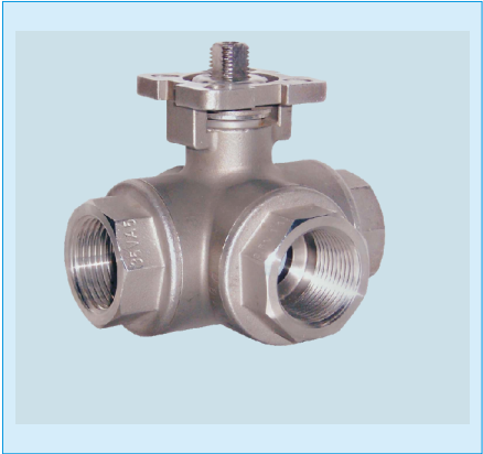
三通, 螺纹端, 1000WOG, 高平台, 减流量球阀 Three ways, F/F threading, ISO5211 pad direct, reduced bore ball valve
