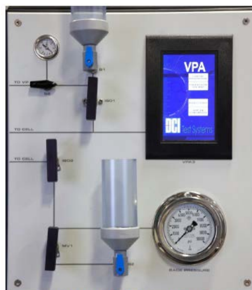
Figure 5: Pore Pressure Control Panel
