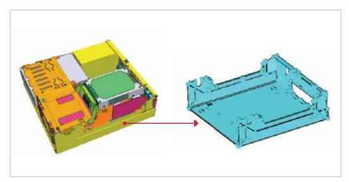
OptiStruct has been used to optimize the structure of a computer case panel and eliminate resonance
