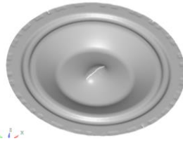
Fig. 15 Crack propagation with MMC fracture model
