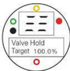
Entire open: red lamp and entire open symbol
