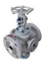
SNY jacketed ball valves are used in the chemical industry for fluids with high viscosity and a tendency to solidify. The valves are designed as a one-piece, fully jacketed unit with insulation media inside the jacket to prevent the solidification of the internal media in the valve, thus ensuring unobstructed flow.
