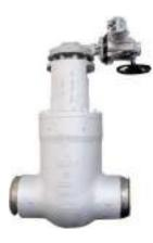
The SNY automated gate valves comply with API 600 and ASME B16.34, and a wider range of products is available for selection, such as pressure seal design, outside yoke and screw, resilient seat design, and bellow construction.
