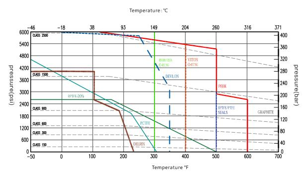
The above chart is for reference only. Please refer to ASME B16.34 for the specific body pressure / temperature rating. Please contact us for specific or additional seat and seal information if required.
