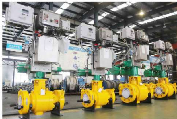
4" 2500# Trunnion Mounted Ball Valve with Hydraulic Actuator
