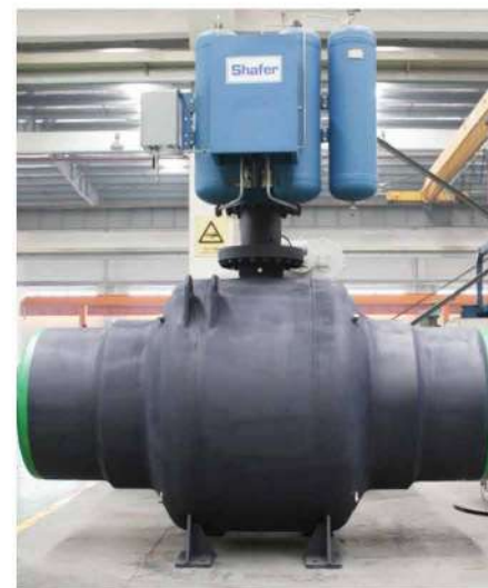
30" #150 Full Welded Ball Valve with Direct Gas Actuator with Local & Remote Operation and line break system
