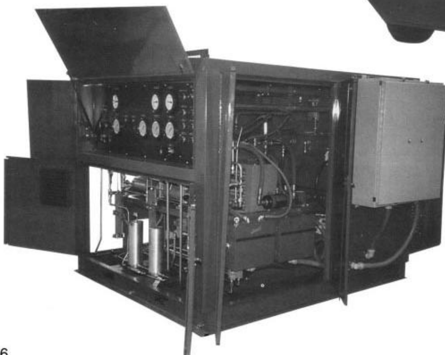
High flow high pressure hydraulic driven helium gas booster system used at many military facilities. Haskel has also introduced a standard line of hydraulic driven gas boosters for industrial applications. (Further details on request).
