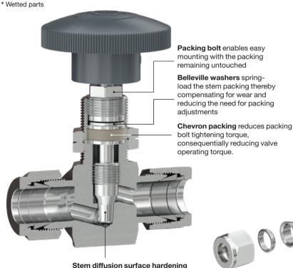
Stem diffusion surface hardening provides the best galling resistance and protection from wear and corrosion.
