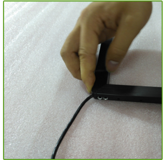
14.Until the whole corner piece has been put into the frame body,be careful not to let the cable out.
