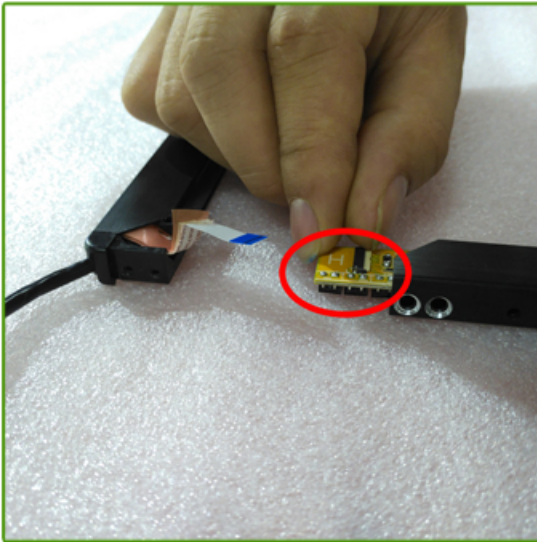
7.Firstly,mount A-A, pay attention to mount the touch frame face up, take out a piece of PCBA.
