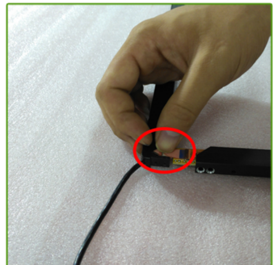
12.Put the FFC cable which have been folded into the groove of the corner piece gently.
