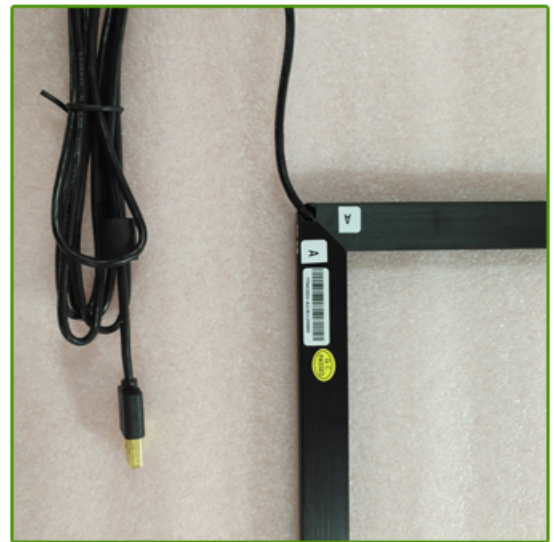
16.The mounting of A-A has been finished,install B-B,C-C,D-D in turn by above methods.
