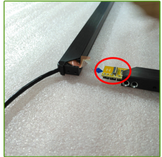
8.As shown in Figure, the buckle of card connector must be standing up, otherwise the touch frame will not be able to insert the FFC cable.
