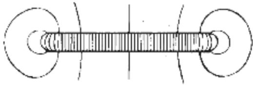
FIG. 6 Flux Lines Between Unguarded Electrodes
