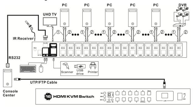
Note: ① HDMI cable ② USB type A to type B cable.
