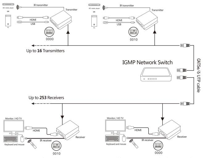
(By using IGMP network switch, support up to 16 transmitters (Addr: 0000~1111) in one local area network. Set the receivers' IP address to the same as the transmitter which the receiver wants to connect to.)
