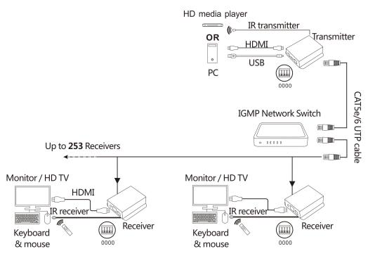
(Set IP address of the transmitter and receivers to the same)
