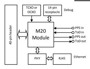
The Development Kit is designed for an optimized IEEE I588 communication application and the Grandmaster mode. The kit is delivered with an on board TCXO, but can be adapted for different oscillators on-board or using an external fixed frequency oscillator. The kit has an optional input for an external reference (eg. GPS).
