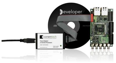
The DK4 development kit incorporates the P40 OEM system with the same general functions as of the DK5/P50, but for a single channel application. The DK4 dimensions are 85x54 mm.
