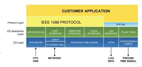
precise time can be used by the software, or, directly by external hardware through the many GPIO ports of the device. The time signal presentation to the external is very precise, since it has no jitter caused by instruction execution.
