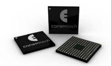
The C34 is an Application Specific controller for time and frequency synchronized applications. Its outstanding features stem from the ability to analyze and act on gate level, in real-time. The central functionality of the integrated circuit is delivered by its hardware based TimeStamp Engine (TSE). The component integrates an advanced operating system environment which enables software to access the timestamping process in a flexible way.
