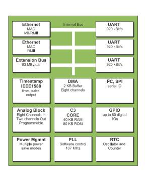
The diagram shows the main parts of the processor. The ROM and RAM memories of the C3 core contain microcode. This enables acceleration of CPU intensive tasks with orders of magnitude.
