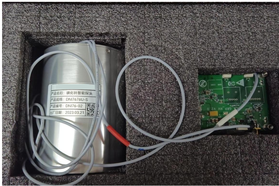
Figure 23 inch sodium iodide intelligent probe (customized product) physical image
