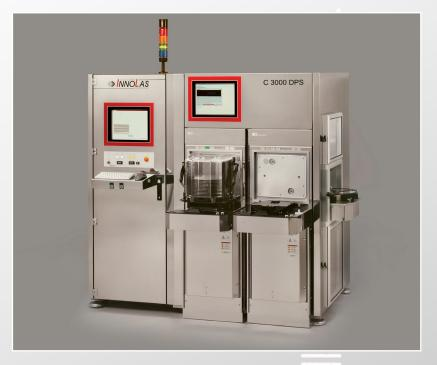
The unique InnoLas Semiconductor designed 300mm vacuum or edge grip handling (including aligner) is available. The system offers marking capability on the front and/or backside of the wafer.
