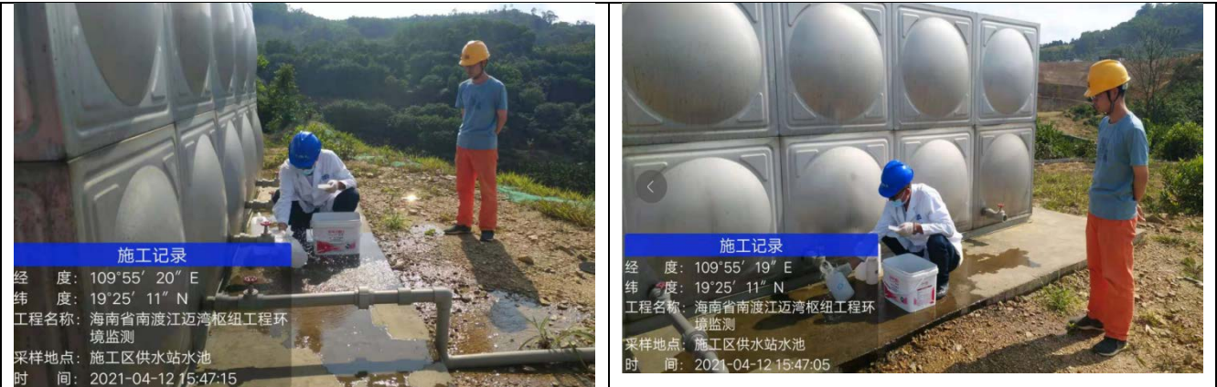
(2021.04.12) 施工区供水站水池饮用水采样
