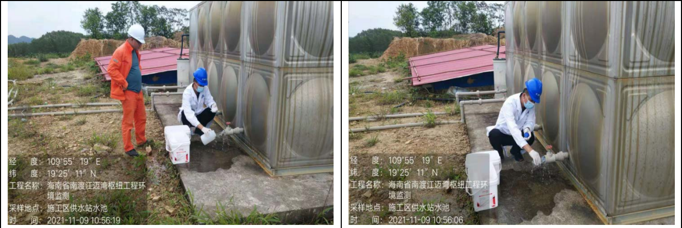
(2021.11.09) 施工区供水站水池饮用水采样
