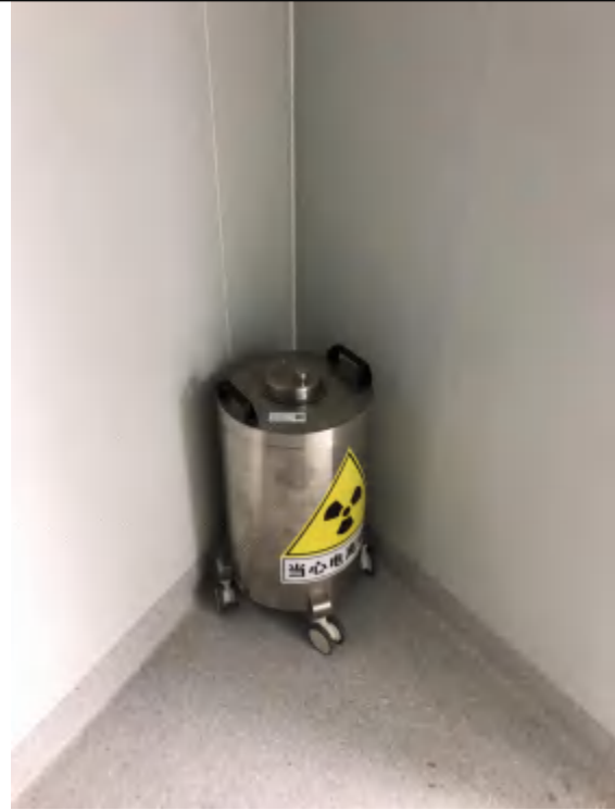
固废间铅废物桶
