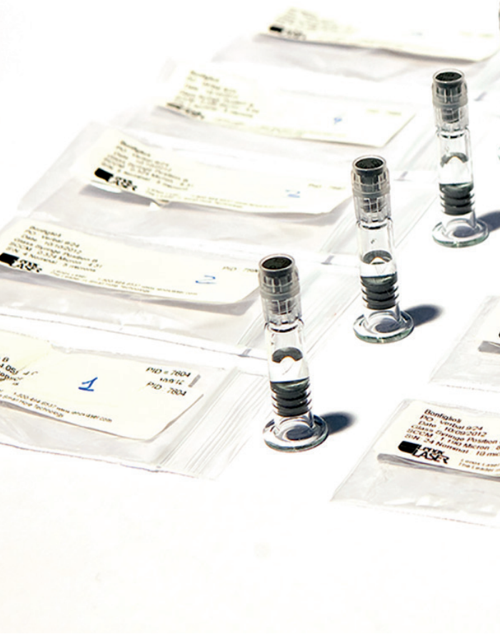
Figure 10 - Complete set of laser-drilled Pre-filled Syringes used for the case study
