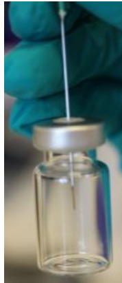
Withdraw 21G needle with capillary remaining in vial
