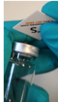
Cut capillary to final total length of <1.5 cm
