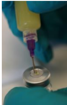
Apply glue around capillary on stopper surface
