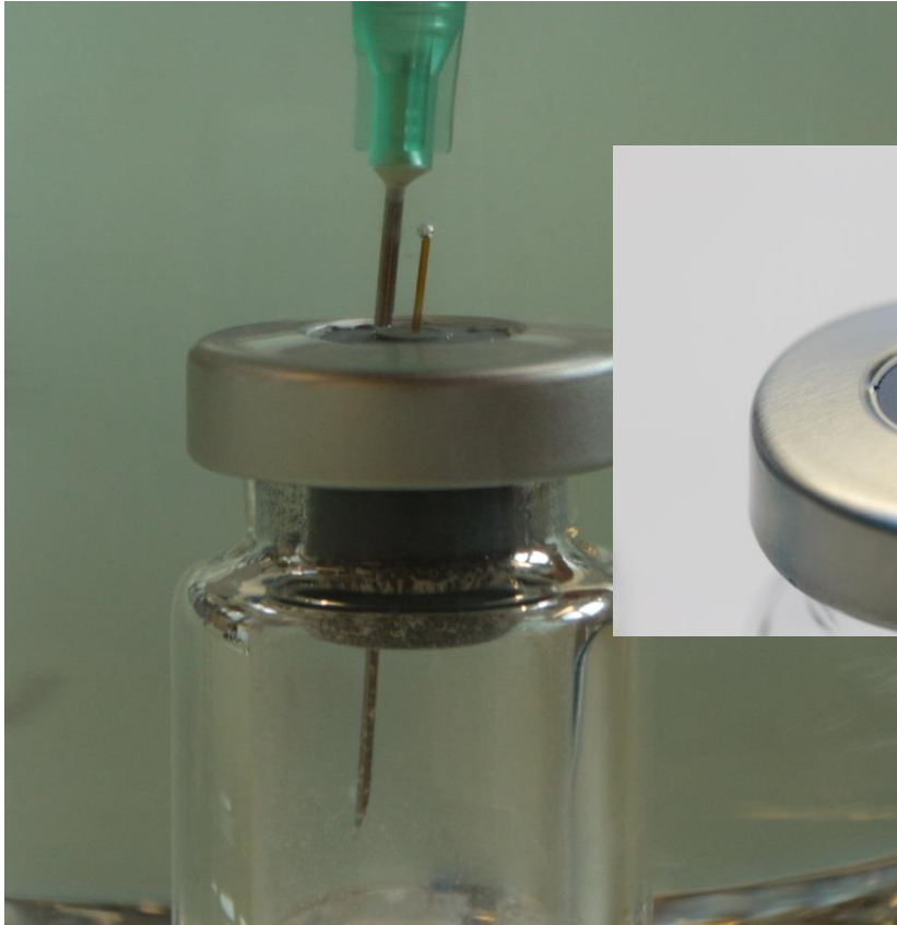
10 \mu m Capillary glued Only defined leakage
