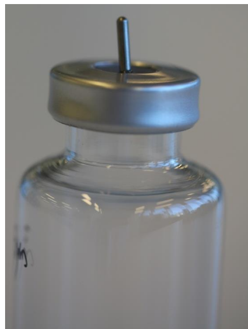
Laser drilled hole in stainless steel capillary which is glued into rubber stopper of a vial
