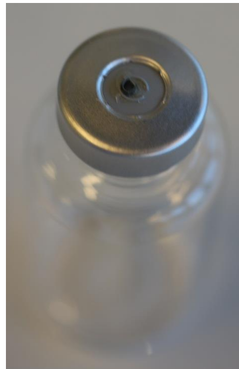
Cut steel needle of 1.6 mm ID glued into rubber stopper
