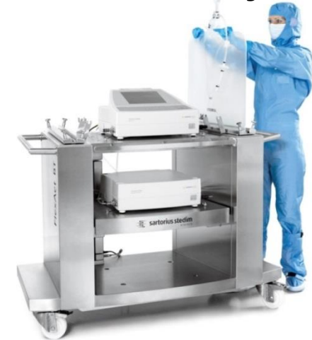
FlexAct® BT Sartocheck® 4 Plus Bag tester
