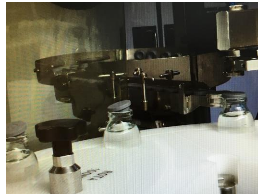
Stopper Insertion Problems Due to Lack of sufficient Lubricity
