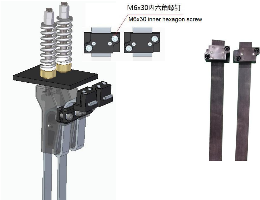
Installation diagram of short-circuit end cutter head
