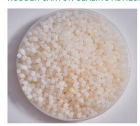
Used temperature: 140°C -170°C Pressure: 2-4 bar
