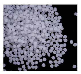
Used temperature: 150°C -180°C Pressure: 2-4 bar
