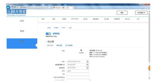
After connected, "network - Interface - PPPO" will start timing "running time", and statistics traffic. can also check network connection status in "Network - Interface Overview" and "Status - Overview".
