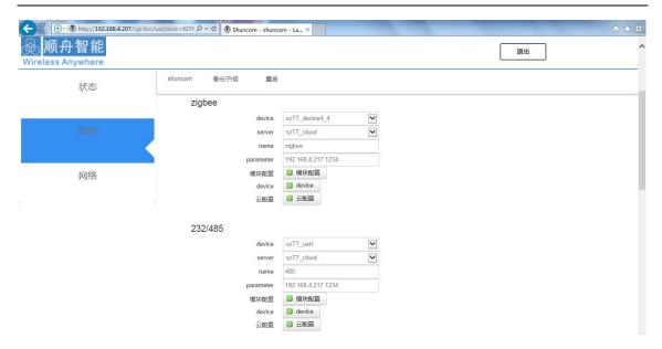
**device:** szTT\_device4\_4 (Zigbee Downlink transparent transmission, With the Shuncom version 4.4 transparent program to use)
