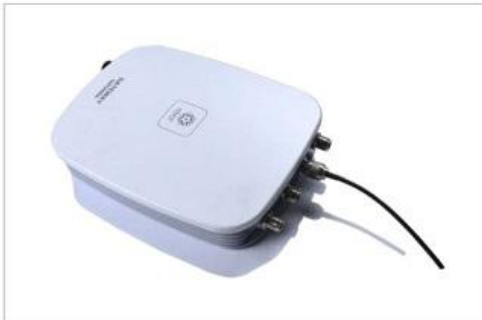
5. Insert the LoRa feeder with one end into the LoRa port, the other end to LoRa antenna with sleeve
