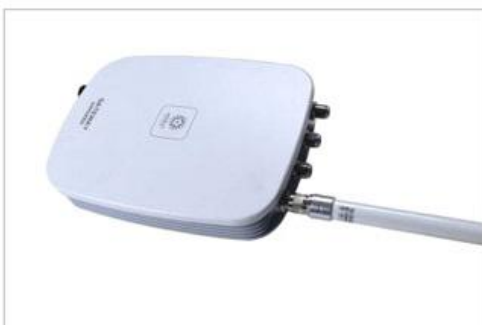
7. Install the Wifi, 4G, GPS antennas into their port, and tighten them
