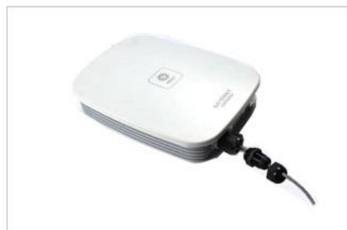
8. Pass the network cable through the RJ45 waterproof rubber ring, press the crystal head, insert the RJ45, and tighten the waterproof ring.
