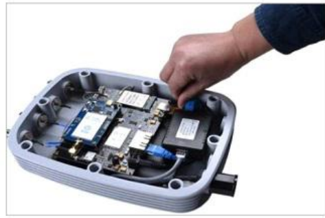
2. Insert the 4G SIM card (Telecom or Unicom or China Mobile) into the card slot (under TF card slot) with the chip outwards and the notch inwards.
