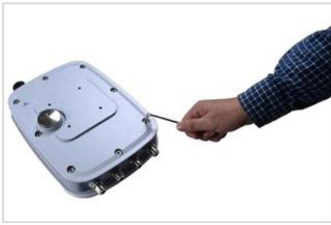
1. Using the hexagonal wrench to unscrew the eight screws on the back of the gateway router.
