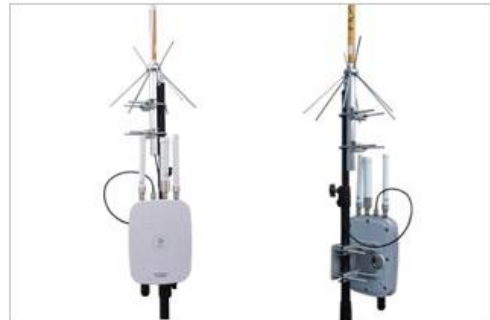
6. Install the gateway with LoRa antenna to the bracket using the holding rod.
