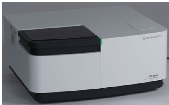
图 1 荧光分光光度计 RF-6000 RF-6000 Spectrofluorophotometer
