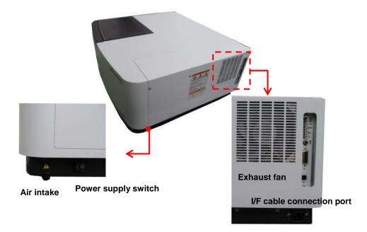
(5) There is a cooling air intake on the left side of the instrument. Leave a space of at least 50 mm between the left side of the instrument and the wall.
