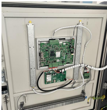
3-7 Check the aging and wear of the charging cable and winding tube
