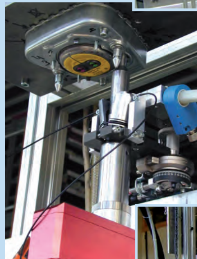
Attaching air bag assembly, vertically from below
