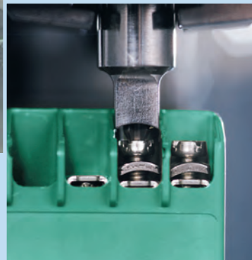
Screwdriver with feeder track for cable clamp screws or heavy-headed screws
