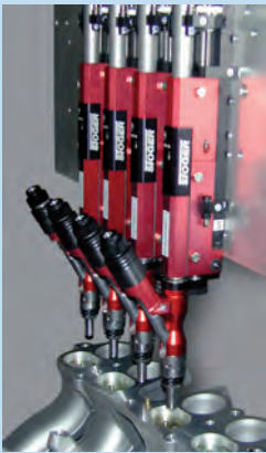
4-spindle screwdriver station
