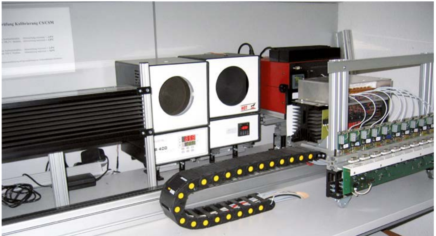
Automated calibration stations at Optris GmbH
