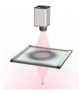
overall system comes with an absolute radiometric calibration traceable to national standards (PTB). To verify compliance of the DUT with IEC laser safety standards, the VTC 2400 enables identification of the maximum intensity spot of the emission pattern.
