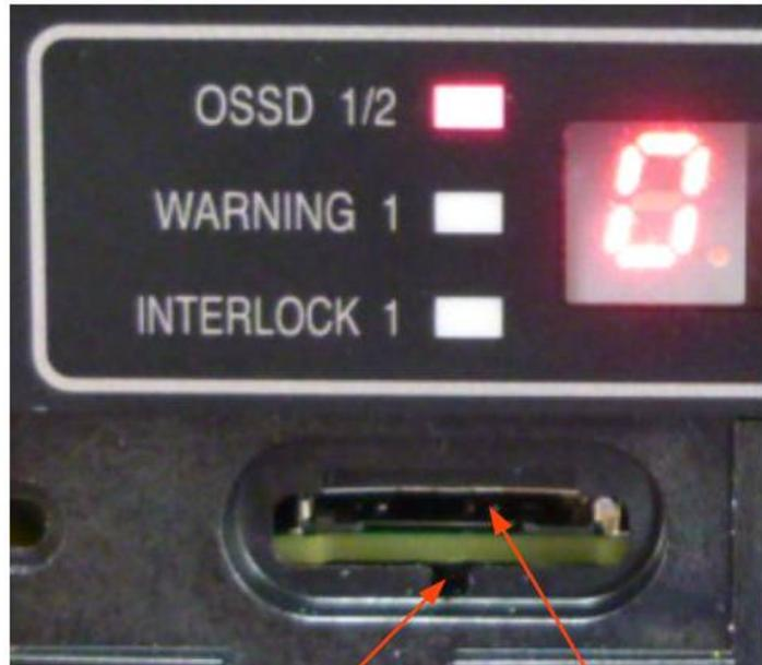
IP Initialization switch      SD Card Insert Slot
