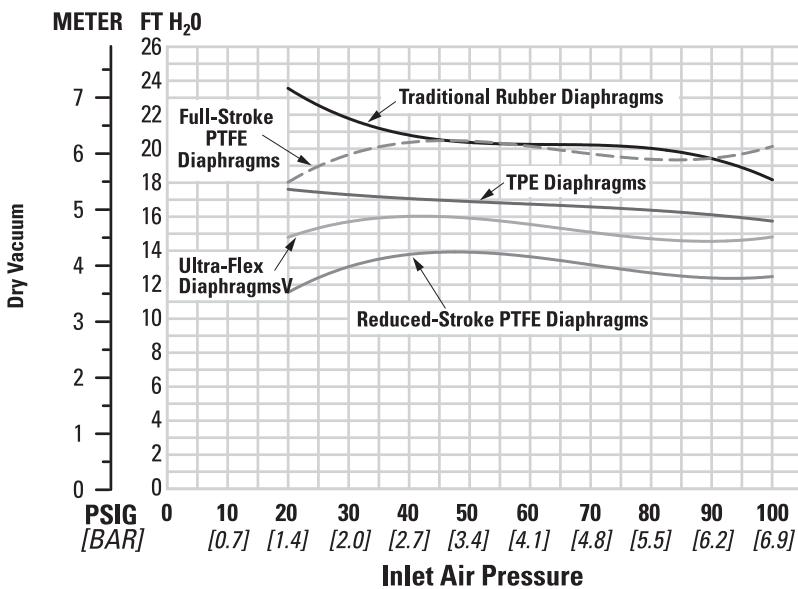
The P8 pump has a 51 mm (2") inlet and 51 mm (2") outlet and is designed for flows to 587 lpm (155 gpm). The P8 pump is manufactured with wetted parts of pure, unpigmented PVDF or polypropylene. A variety of diaphragms and O-rings are available to satisfy temperature, chemical compatibility, abrasion and flex concerns.
