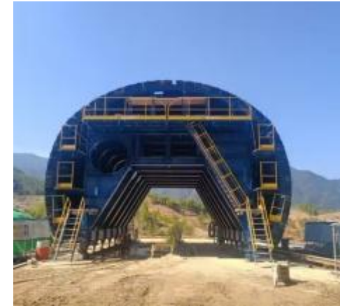
The tunnel layer distributor is used in conjunction with the lining trolley
