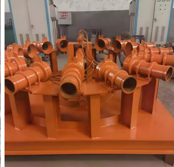
The tunnel layer distributor is used in conjunction with the lining trolley
