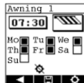
Time and date can be entered in the timer menu. Use the horizontal navigation keys to move the blinking cursor for input either to the left or to the right.
