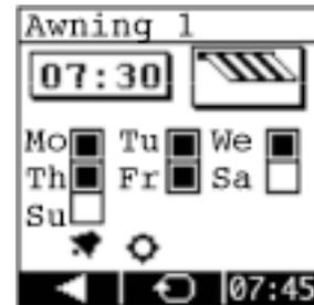
A programmed timer can be disabled without going through the set up menu by using the multifunction key
