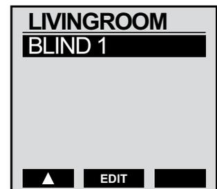
Should another actuator be added, press the navigation key DOWN
