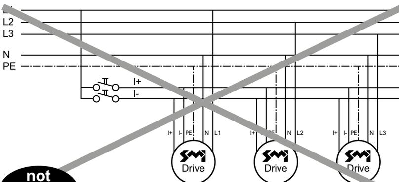
**not permitted** Push button operation with power supply from different phases
