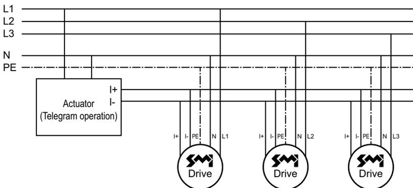
**permitted** Telegram operation with power supply from different phases
