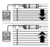
Restart the setting procedure from the beginning to set an end position again! The lower or upper end positions can also be detected automatically (sets to torque) and taught in!
