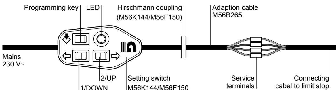
**Connection with setting switch M56F151 with service terminals**
