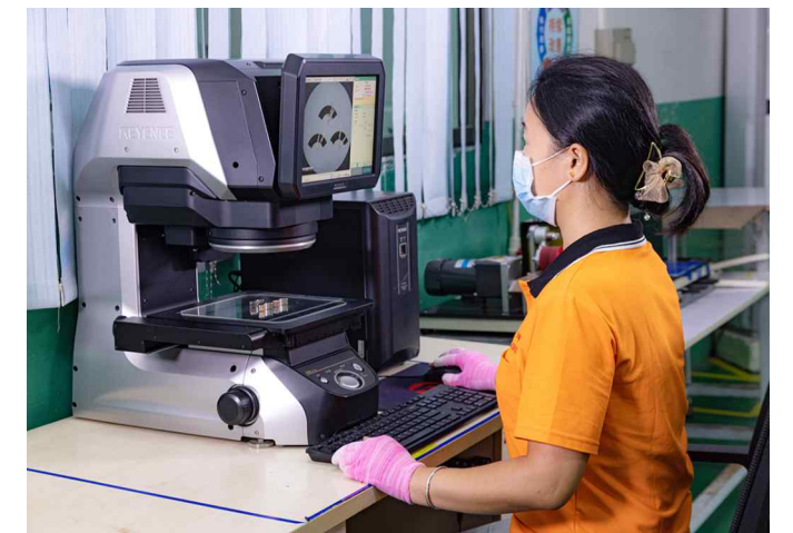
二次元投影检测 Binary projector inspection
