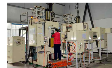
全自动磁场成型压机 Automatic magnetic field compression molding machine
