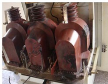
Fig. 5.2B PT Insulation Breakdown Failure
