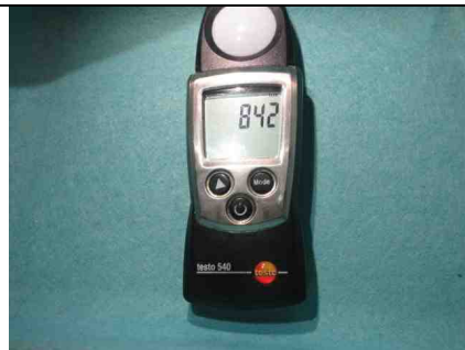
47) 842 lux at final inspection station
