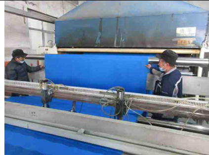
17) 100% inspection station after weaving
