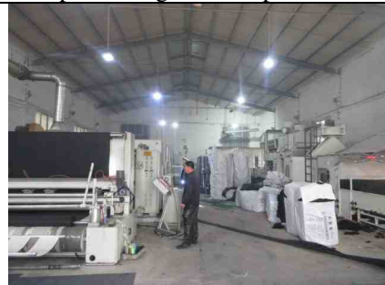
23) 3 rd workshop for front processing (polyester fiber loosing, mixing, carding and weaving)
