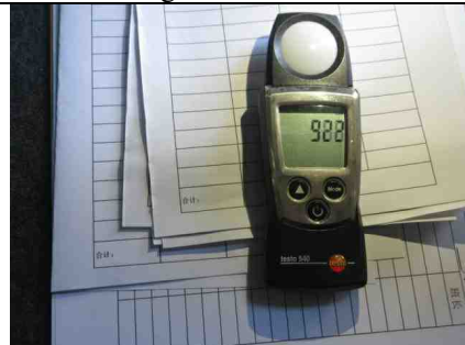
20) 922 lux at IPQC station in front processing workshop
