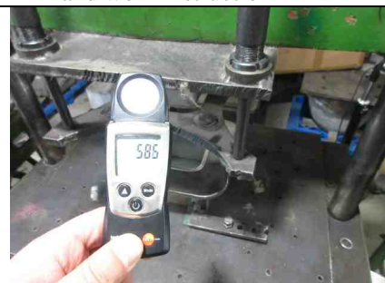
35) 585 lux at hot press forming workstation
