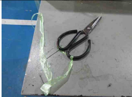
16) Fastened sharp tools at weaving workstation
